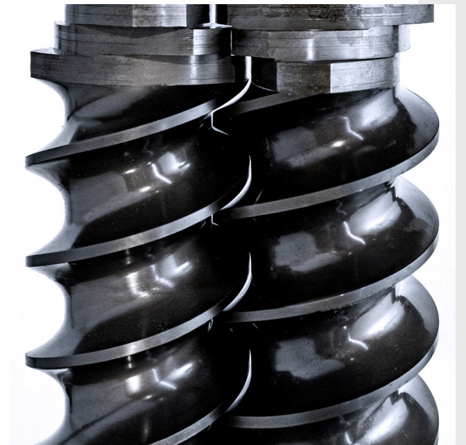
Two co-rotating screws composed of modular sectors.
