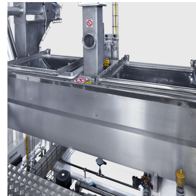
Mixing tank ensures proper kneading and cooling time for the cooked dough.
