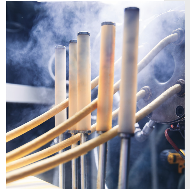
Cooking Extrusion Head of a GEA xTru Twin 70 cooking extruder installed on a pillows processing line.
